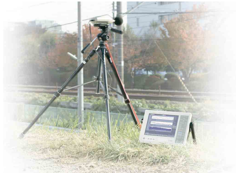
Outdoor noise analysis using the CF-7200 and an LA Series Sound Level Meter
