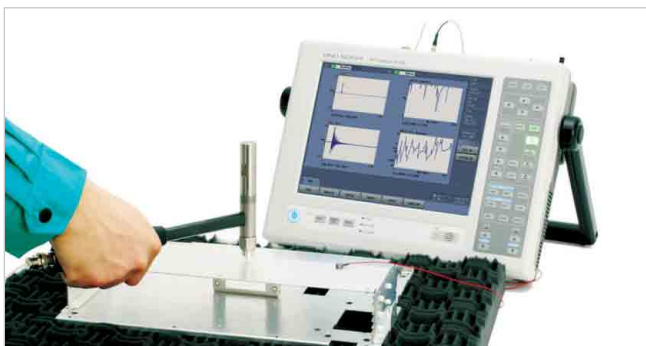
Hammering measurement with the CF-7200, GK-3100 Impulse Hammer and an NP Series Acceleration pickup
