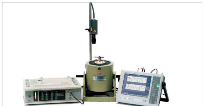
Analysis of micro-object using a LV Series Laser Doppler Vibration Meter and an electromagnetic shaker
