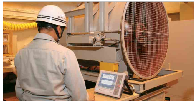
Rotational vibration measurement of a large blower using the CF-7200
